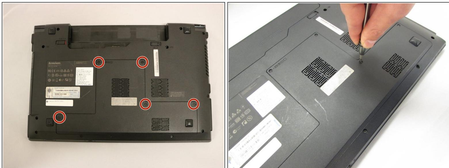
*(i)* The screws are captive to the back panel so they are not to be removed.
