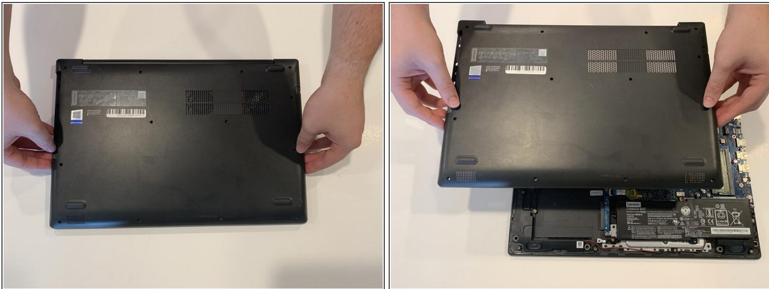
**ⓘ** Make sure that the back panel is completely free from the laptop.
