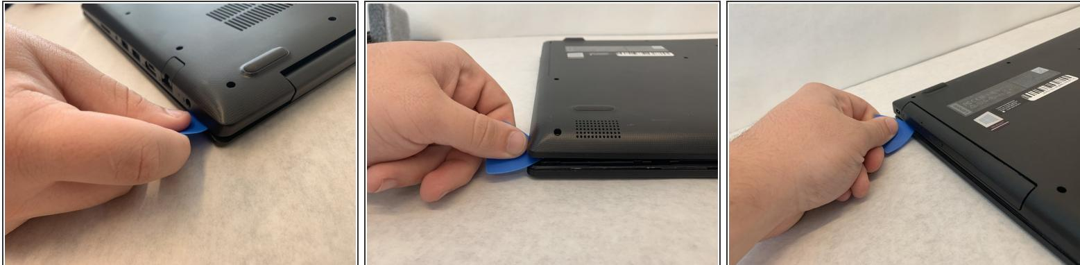
**⚠** Do not try to completely remove this case without ensuring the entire case is free of connection points as this could crack or damage the case.
