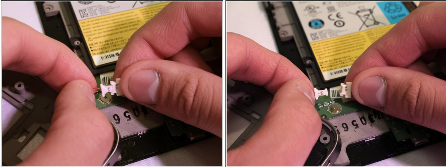
*(i)* The speaker in the grey frame is connected to the motherboard by the white plastic connector.
