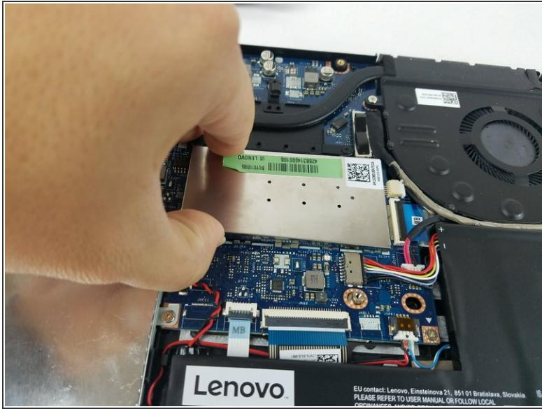
**⚠** RAM cards can be damaged from exposure to a static charge through contact with the hand or other body parts. Though the damage of one discharge is not severe, multiple exposures can cause your RAM to fail.
