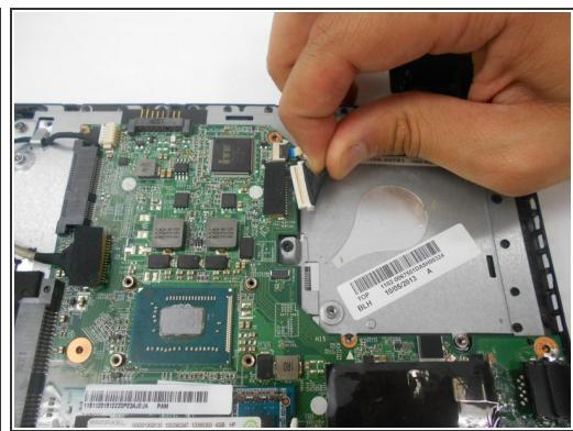
*(i)* Your device may or may not have tape securing wired connections. If it is present, it must be removed before disconnecting cabling.
