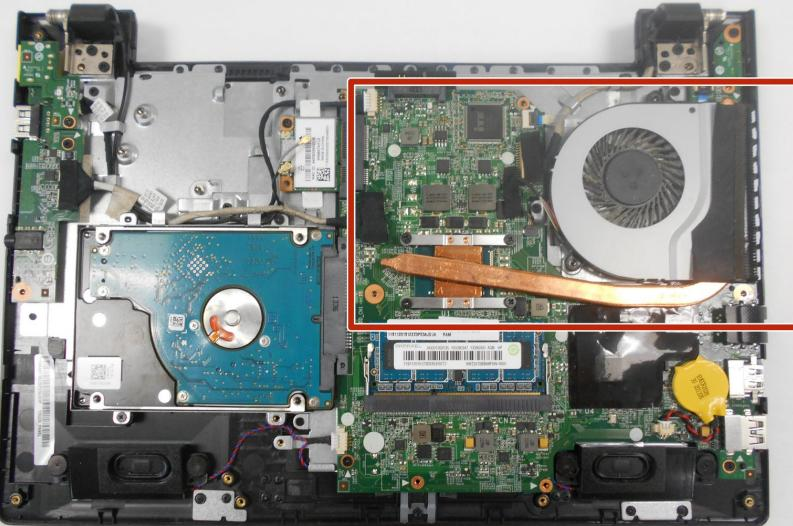
*(i)* Many of the wire connections to the motherboard are secured by tape for vibration protection. Your device may or may not have this tape.
