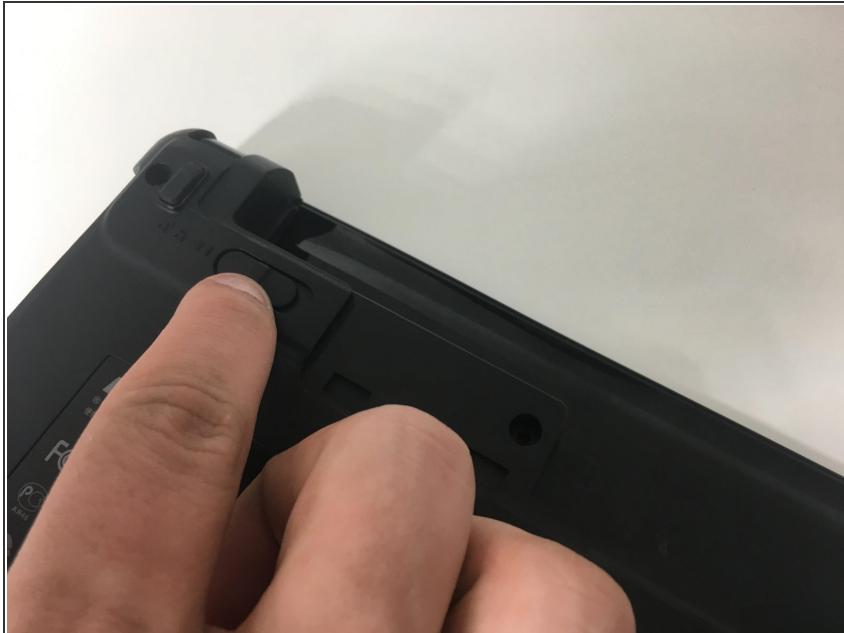
i On the top left of the laptop there is a switch. Make sure it's pushed in the unlocked position.
