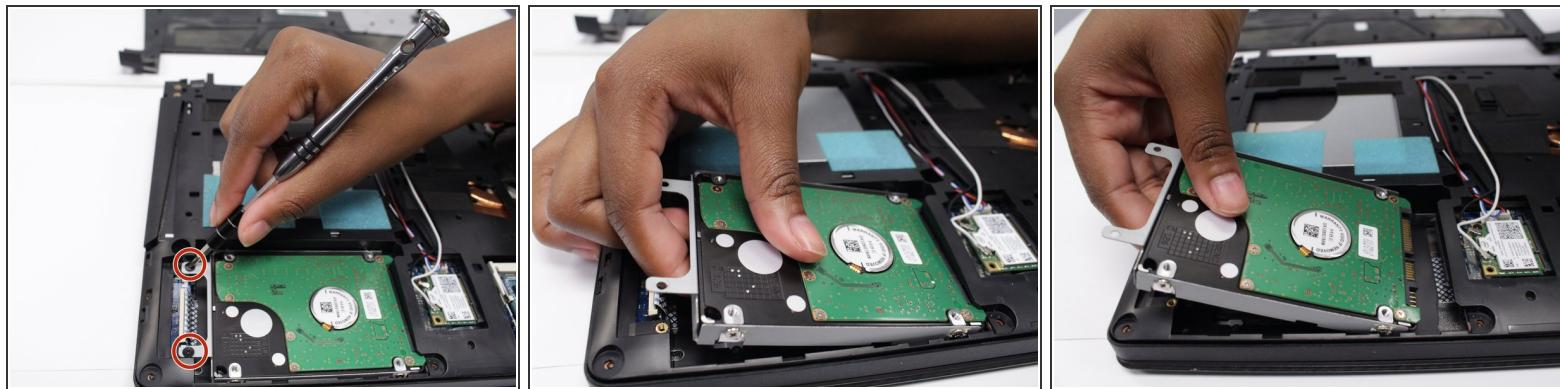
**⚠** If you intend to reuse this hard drive, be careful removing it as hard impacts may damage the device.
