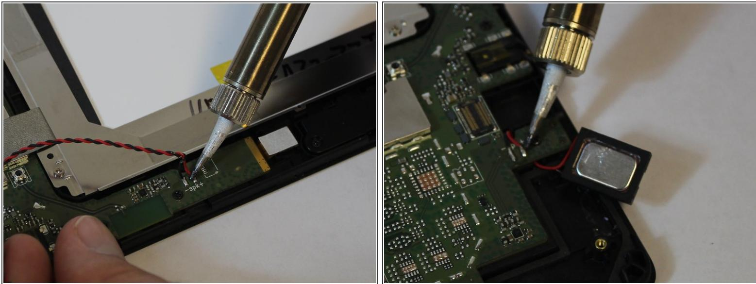
*(i)* This step is not necessary if you aren't replacing the speakers.
