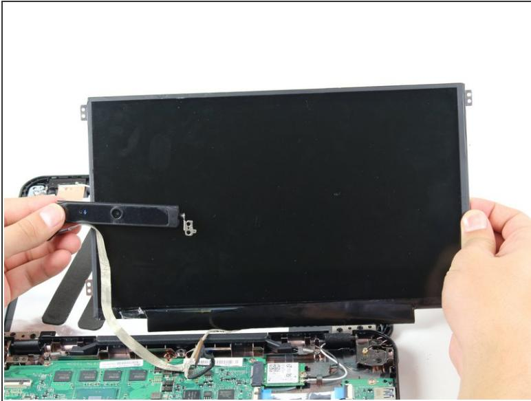
**⚠** When you lift the screen and camera out of the back casing there will be an adhesive that keeps the screen and camera attached to the metal panel. Lift the screen slowly so you do not damage the metal panel or screen.
