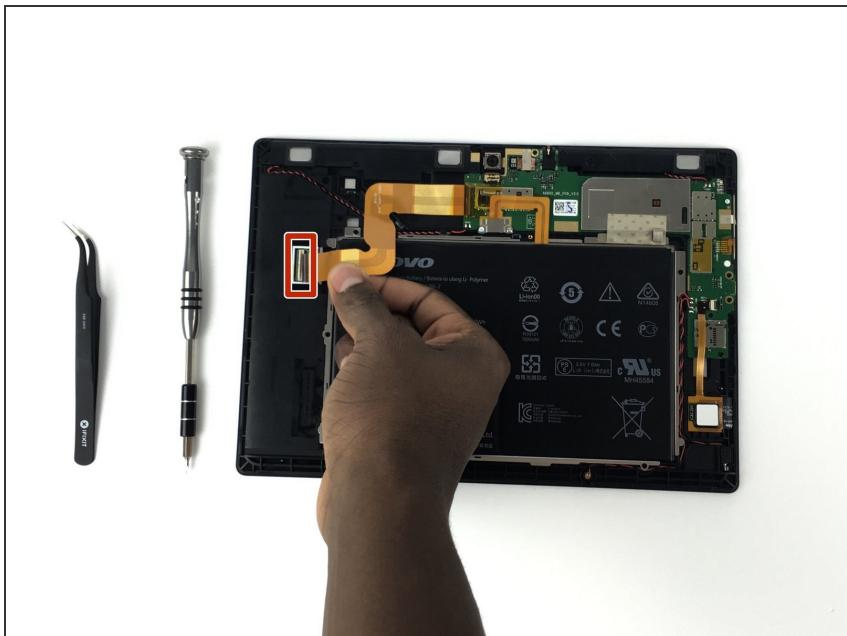
**⚠ Handle ribbon cables with care so it does not rip or tear.**
