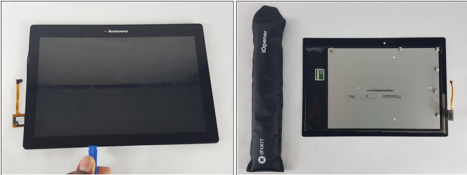
*(i)* The screen is secured by adhesive around all the edges of the screen.
