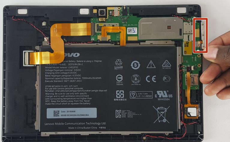
*(i)* The power button strip is only held in place by a small piece of double-sided tape.
