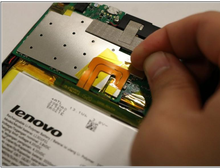
*(i)* The battery is connected to the motherboard by the thin wire shown here.
