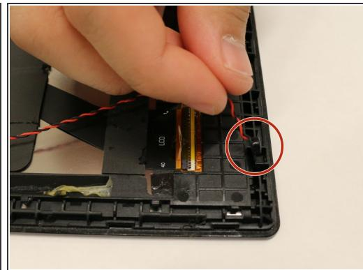
**ⓘ** There are two twisted pairs of wires on the left and right edges of the case.
