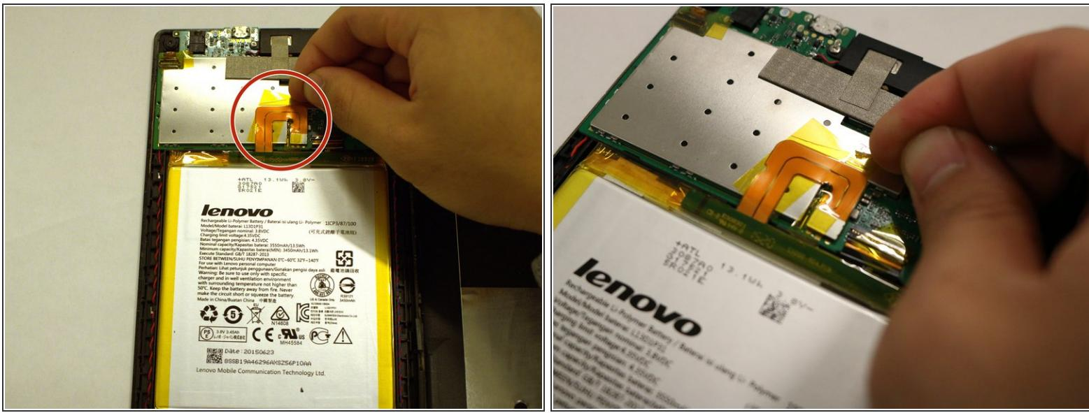
① The battery is connected to the motherboard by the thin wire shown here.
