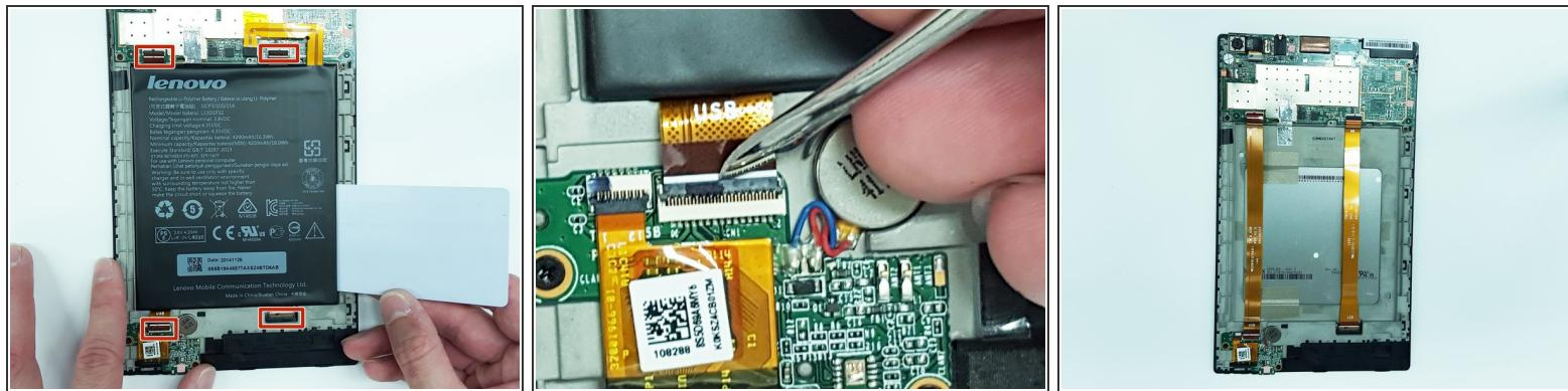
**⚠** The ribbon cables under the battery need to be detached from other electronics as a precaution in case the ribbon cables remain stuck to the battery during removal.
