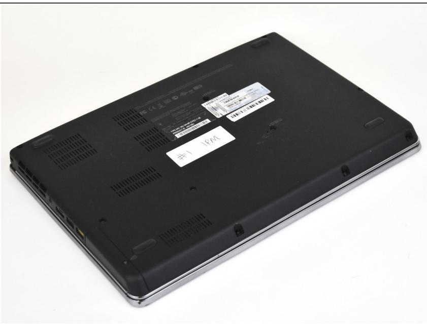
⚠ There is no external access to the battery. Please make sure the battery has been drained or disabled through BIOS before beginning.
