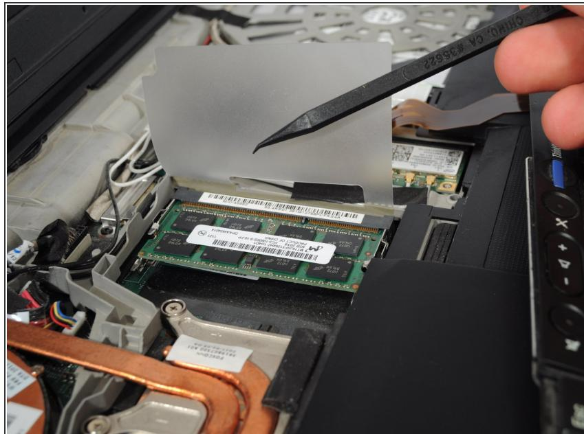
ⓘ Here is your second chance to modify your RAM configuration. As before, there are two DDR3 SDRAM slots. Here they are stacked on each other, not side by side like the bottom. You may install up to 8 GB in each slot, allowing for 16 GB of RAM total.
