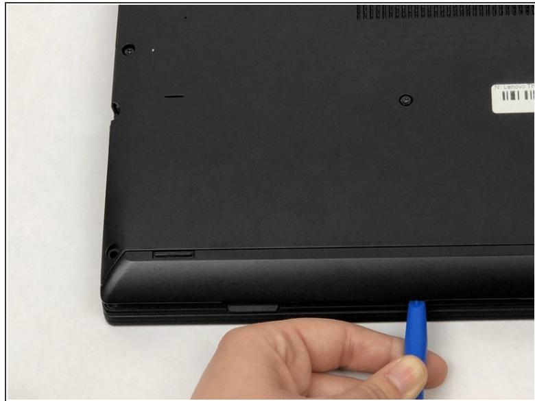
ⓘ The bottom cover is attached via several plastic clips located around the edges of the bottom cover.
