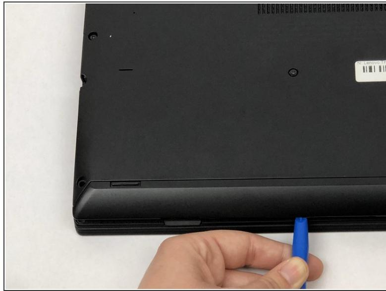
*(i)* The bottom cover is attached via several plastic clips located around the edges of the bottom cover.
