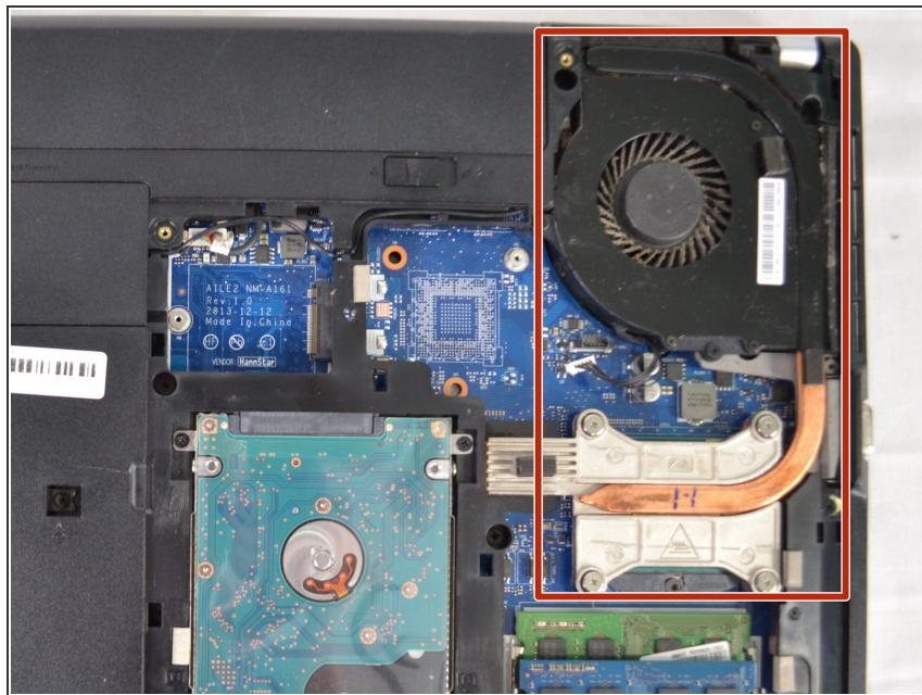
*i* Heatsink and fan are connected. You have to remove both at the same time.
