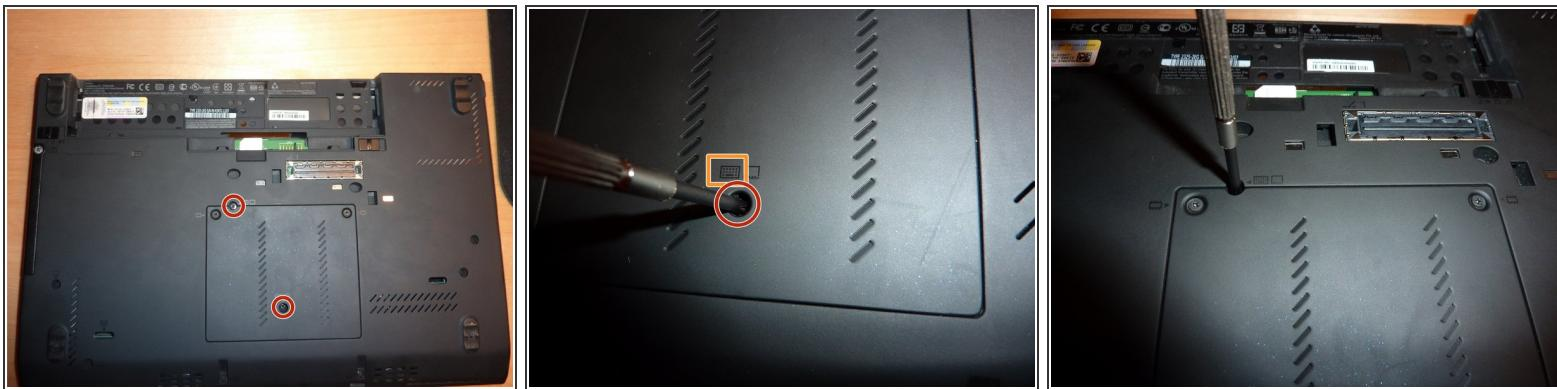
*(i)* There are 2 screws securing the keyboard. You can identify them by a small keyboard symbol (marked by an orange rectangle in the second picture).
