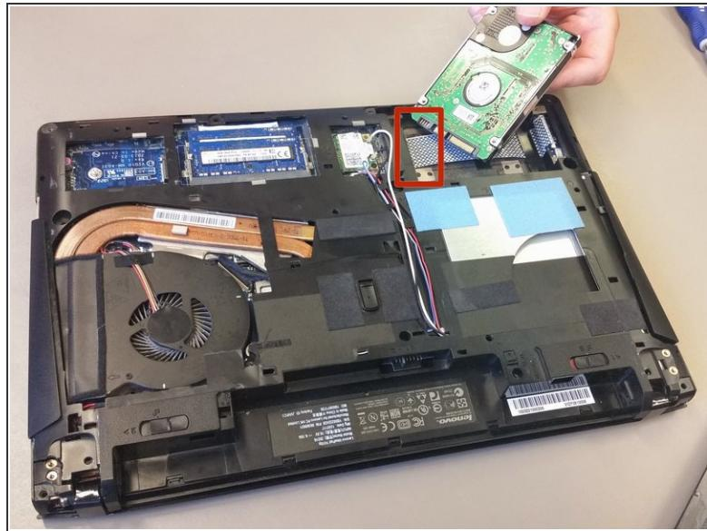
! If you intend to reuse this Hard Drive/SSD, be careful with the removal. Hard impact may result in damage.
