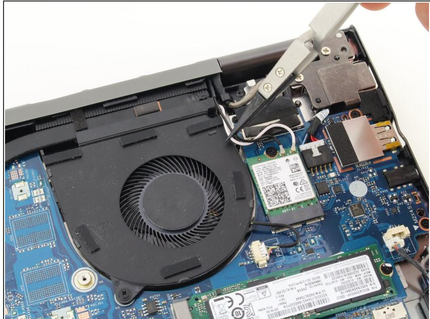
**ℹ** When the laptop is upside down, the left fan is on the right side of the laptop near the wireless card and the SSD.
