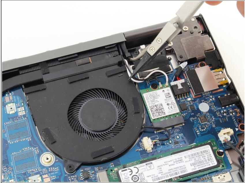
When the laptop is upside down, the left fan is on the right side of the laptop near the wireless card and the SSD.
