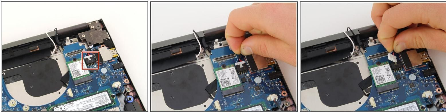
ⓘ The charger port is connected to the computer by a cable at the top left of the motherboard.
