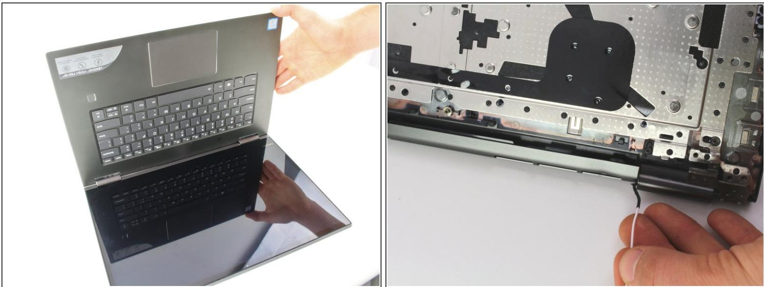
ⓘ Tilt the keyboard up to make a 90 degree angle with the screen. This makes it easier to move the display and antenna cables.
