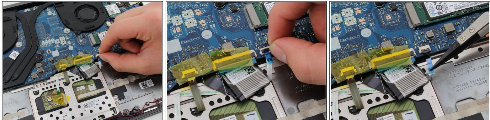
**ⓘ** The touchpad is connected by a ribbon cable to the front edge of the motherboard.
