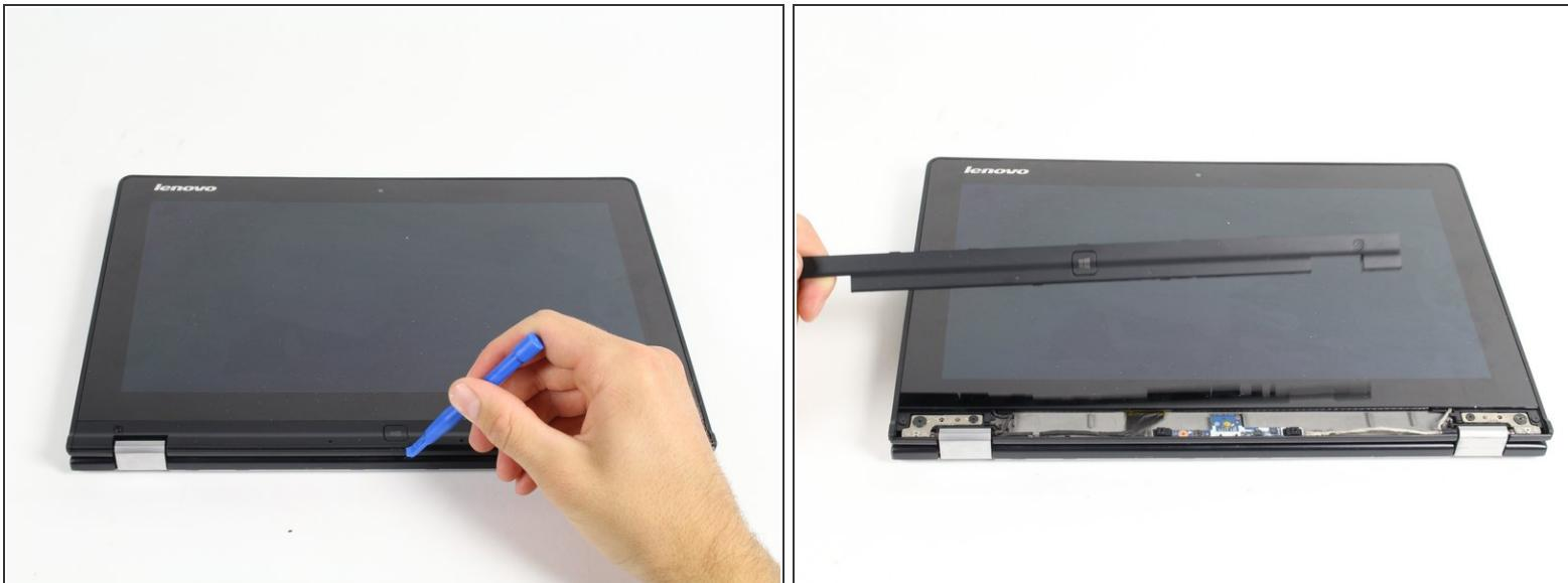
**ⓘ** Flip keyboard under the screen for ease of repair.
