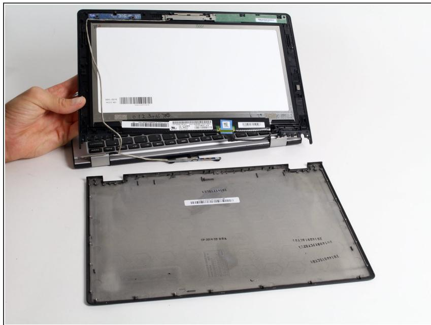
**⚠** Use caution when removing the screen from its back, as the screen is pretty fragile.
