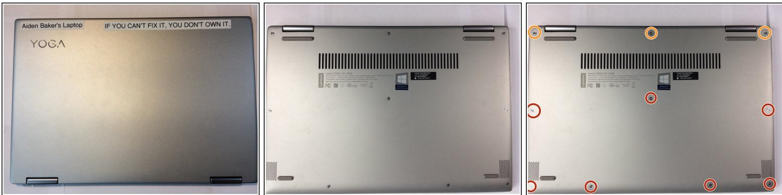
ⓘ Start by flipping the device over so that you see the screws.
