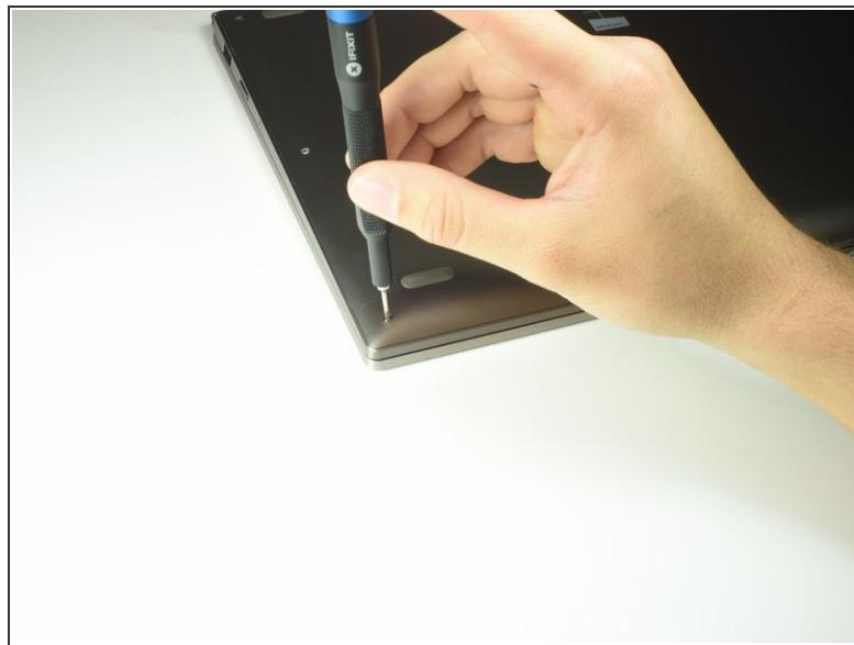
*(i)* Flip the device over to access the screws on the back cover.
