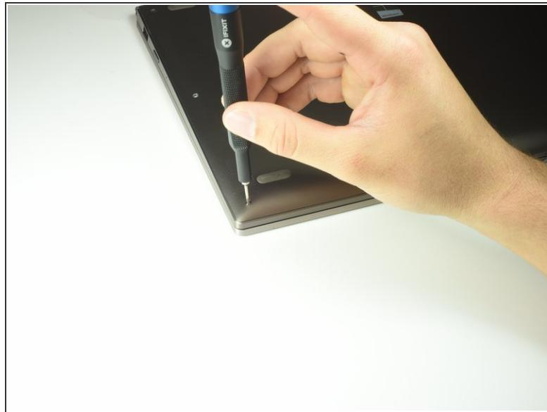
ⓘ Flip the device over to access the screws on the back cover.
