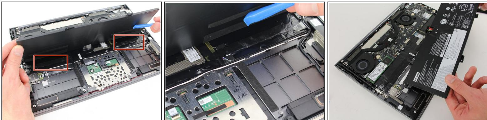
**i** The battery is firmly stuck to the laptop body.
