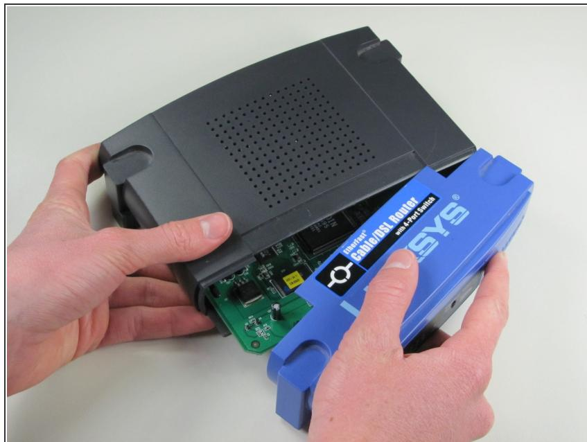
ⓘ There actually aren't any screws or notches under the rubber feet on this model. A little force is all that's needed to pull off the front blue panel. (The front is held on by a recess/notch on each side)
