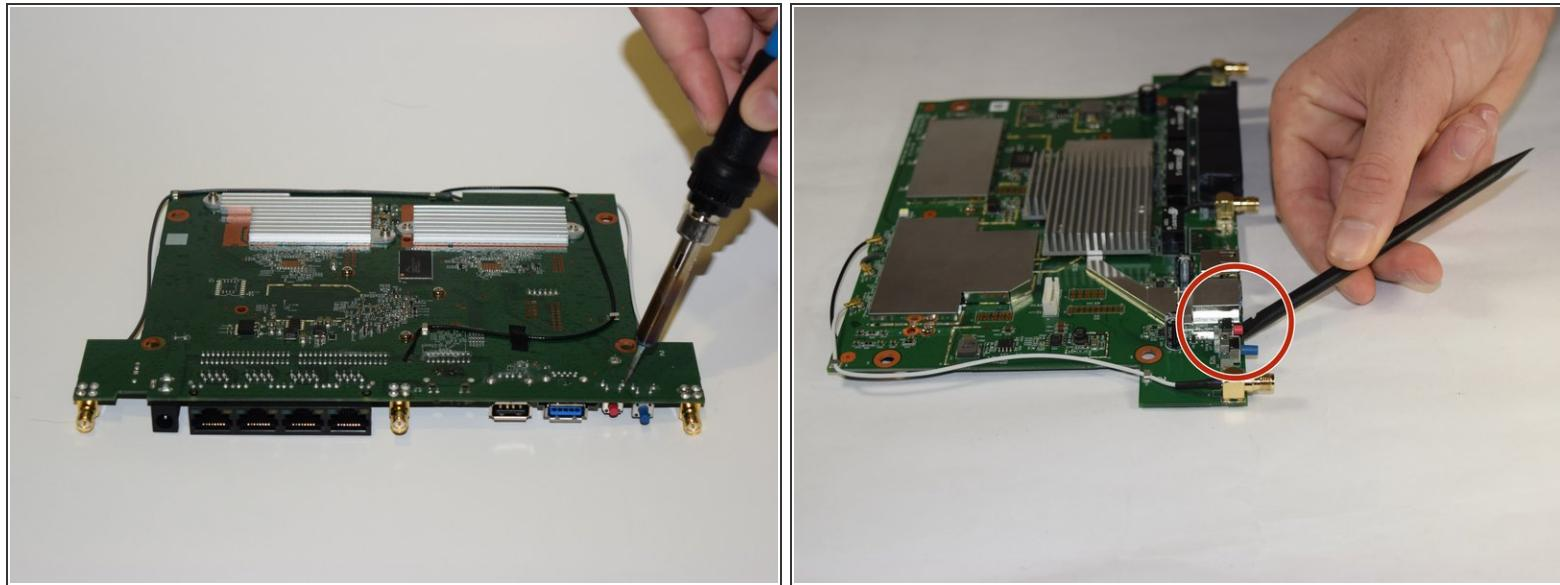
**⚠** Be careful when working with the hot soldering iron! Make sure the router motherboard is safely resting on a level and sturdy surface.
