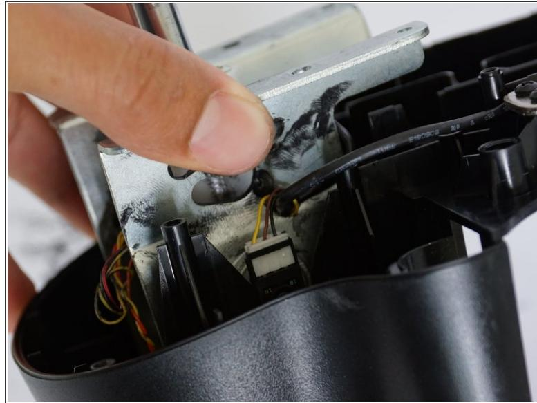
! There is grease covering the whole shifting assembly so it will get messy when removing.
