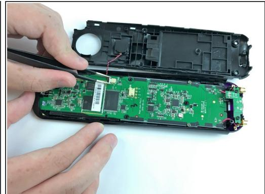
! Carefully remove the back cover and place it next to the remote. Be careful not to detach the wire during this process.
