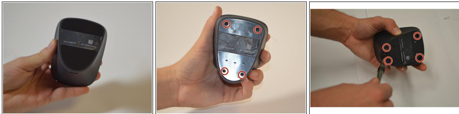
*(i)* Screws are hidden beneath rubber pads.
