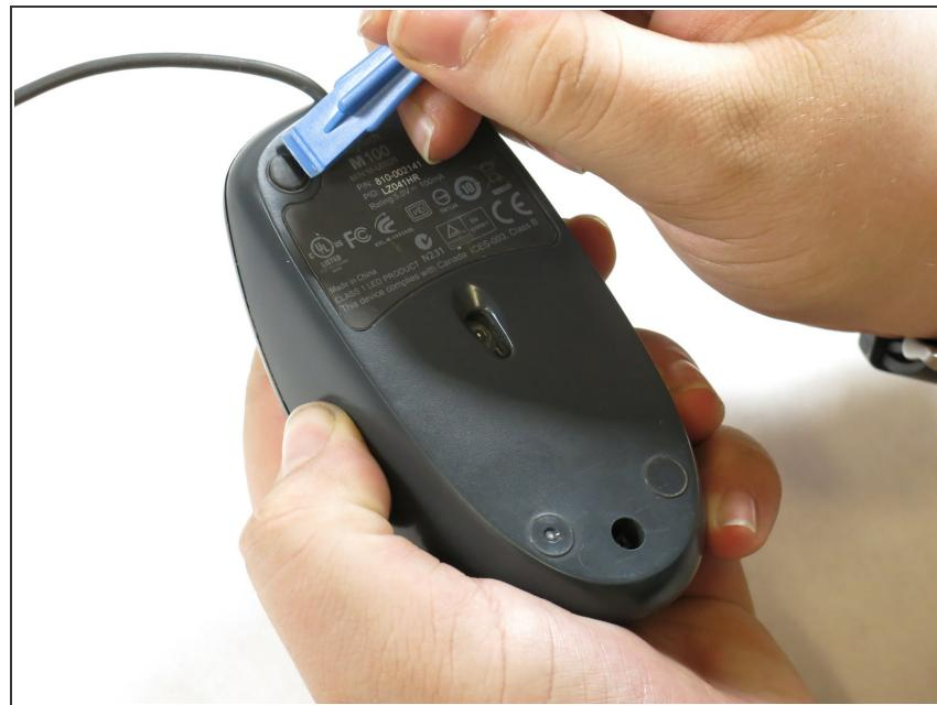
After re-assembling the mouse, don't forget to reattach the mouse feet onto their correct locations on the bottom of the mouse.
