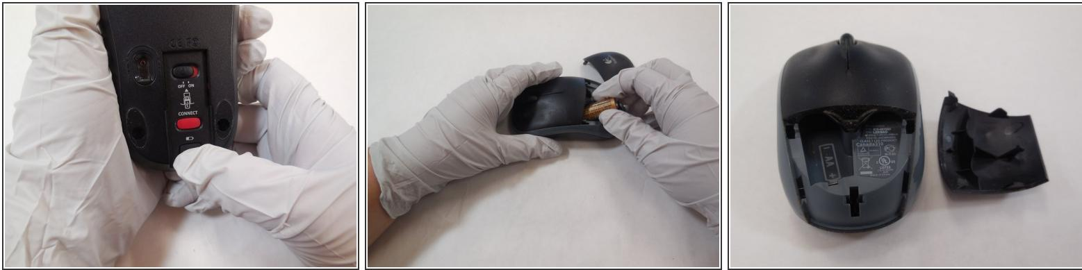
**⚠** Removing the battery ensures that when you get into the circuit board of the mouse, you will not be shocked by any energy coming from the batteries.
