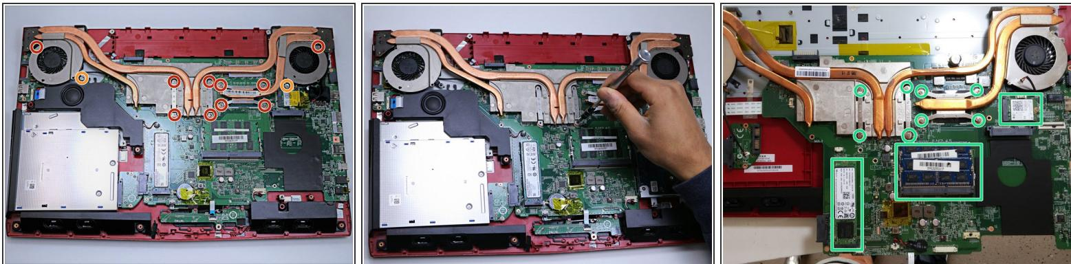
ⓘ If you are replacing only the keyboard, you can skip to step 18, and then skip the WiFi adapter removal step. The CPU fan, m.2 SSD, RAM and WiFi adapter (marked in green) will all come off with the main board, giving you access to the keyboard.
