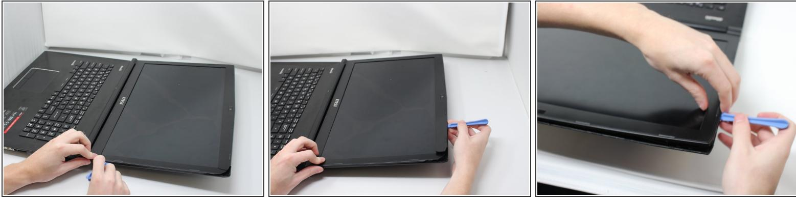
**⚠** Be careful when removing the bezel. The clips that hold it in place will break when too much pressure is applied.
