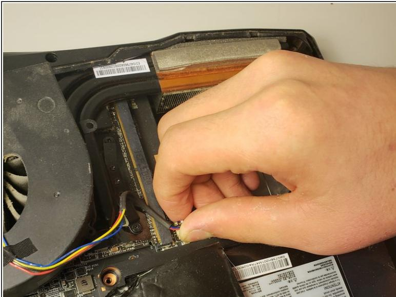
*(i)* The white plastic clip secures the fan wires to the laptop.
