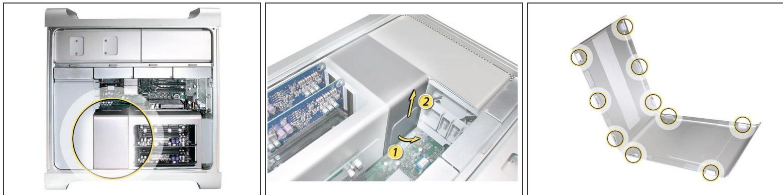
**i** Note: The heatsink cover is held in place by a number of tabs and magnets on the underside of the cover. You must release the tabs before you can remove the cover from the enclosure.
