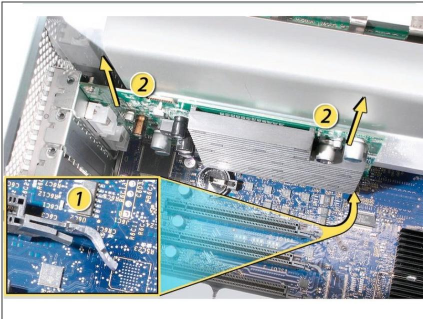
⚠ Warning: When removing or installing a card, handle it only by the edges. Do not touch its connectors or any of the components on the card. Lift the card straight out from the connector to remove it, and insert it straight into the connector to install it. Do not rock the card from side to side and don't force the card into the slot.
