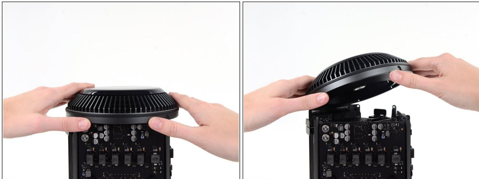
*(i)* The fan assembly is attached to the rest of the computer by two cables on the IO board side.
