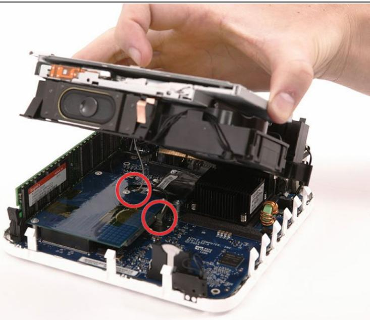
*(i)* If your mini has neither an Airport card nor a Bluetooth board, you can simply lift the optical drive up and away. Otherwise, you need to disconnect the Airport and/or Bluetooth antenna cables first.
