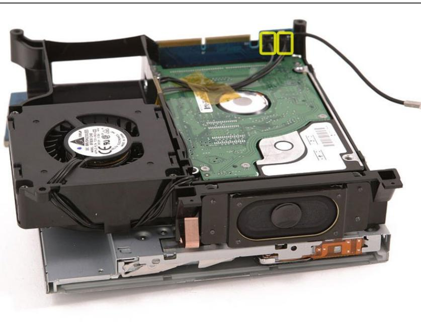
**⚠** The cables you're about to remove are very fragile - do not pull directly on the wires. Instead, try to pry up the connector directly, using your fingernails or a small flathead screwdriver if necessary.
