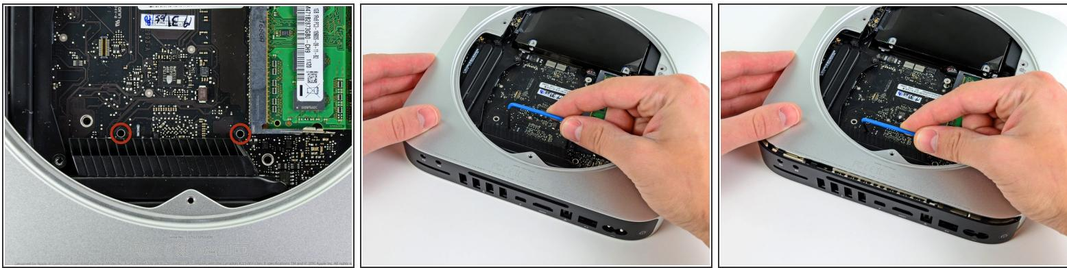
**⚠** To remove the logic board, the two cylindrical rods of the Mac mini Logic Board Removal Tool must be inserted into the holes highlighted in red. Inserting instruments into any logic board holes other than the ones highlighted in red may destroy the logic board.
