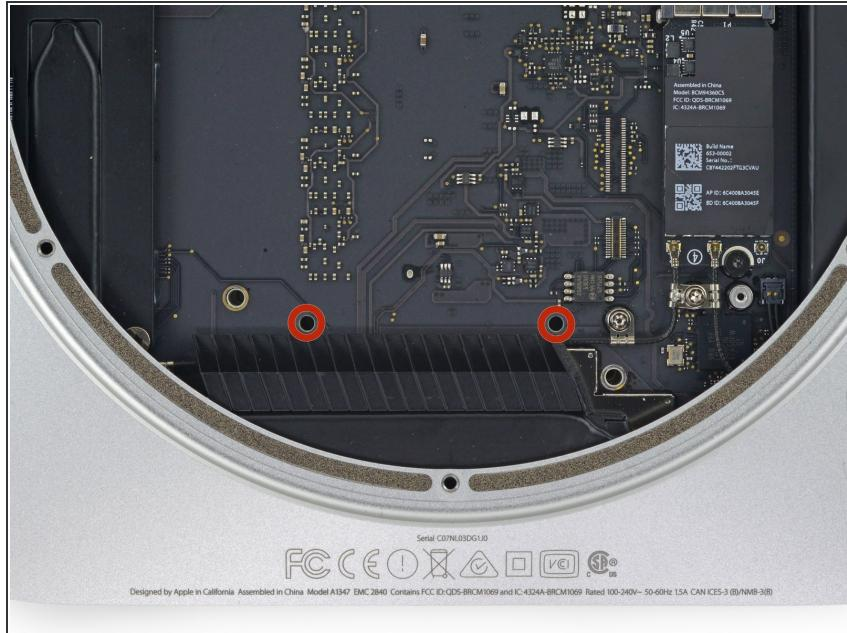
**⚠** To remove the logic board, the two cylindrical rods of the Mac mini Logic Board Removal Tool must be inserted into the holes highlighted in red. Inserting instruments into any logic board holes other than the ones highlighted in red may destroy the logic board.
