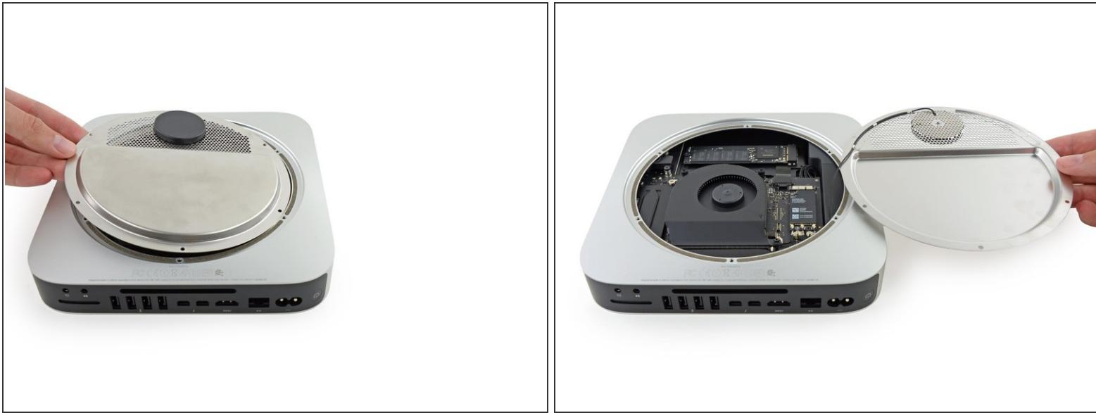
**⚠** Do not completely remove the antenna plate; it is still connected to the Mac mini by an antenna cable.
