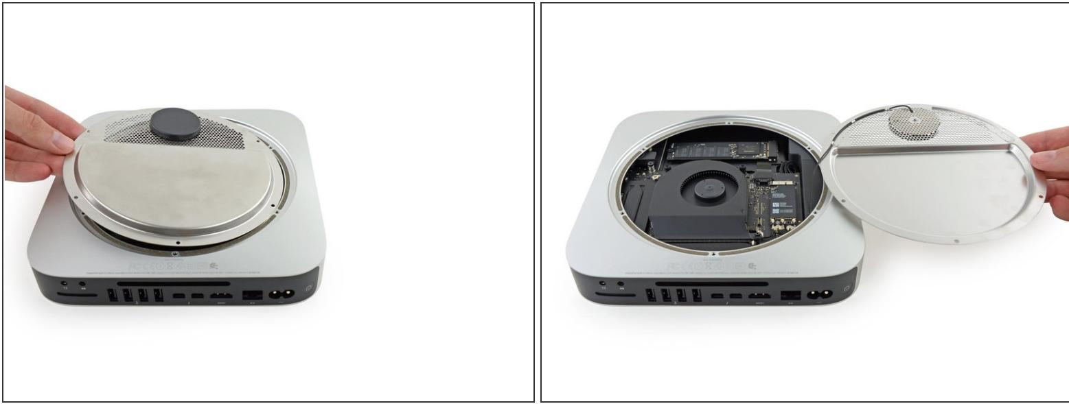
**⚠** Do not completely remove the antenna plate; it is still connected to the Mac mini by an antenna cable.
